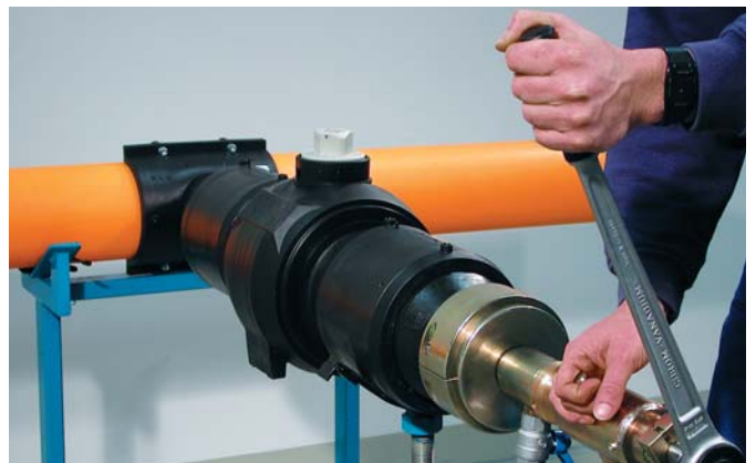
Picture 4: Drilling via clamping fixture and ball valve
