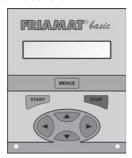
**MENUE:** The MENUE button is grey. It calls up the main menues with the sub menus "Basic settings", "Info" and "Emergency input". In addition pressing the MENUE button will clarify an error following an error message.
