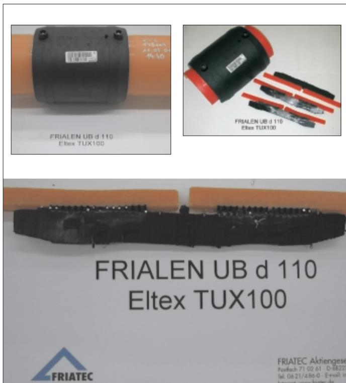
**Fig. 9:** Manuell Folding/Bending test of PE100 Fitting/ TUX100-Pipe: Preparation – Test specimen – Result: Ductile break, high separating forces
