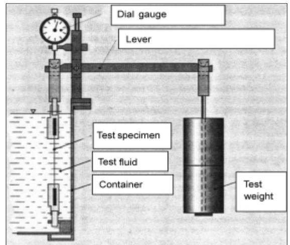
**Fig. 3:** Long term tensile test: Testing method
