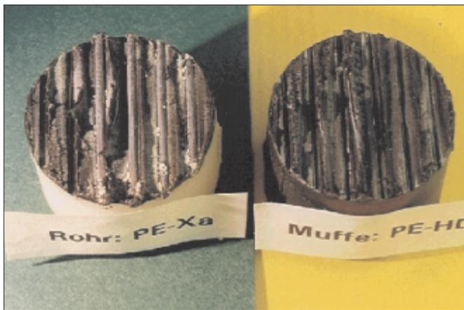
**Fig. 6:** Long term tensile test: Rapture of the joint between PE-Xa-pipe (white, left) and PE100-electrofusion coupler (black, right)
