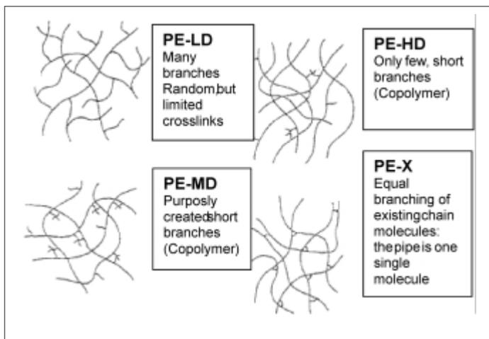
**Fig. 1:** Molecular structure of cross-linked polyethylene compared to LD-PE, MD-PE and HD-PE. Configuration of chain molecules in the amorphous ranges [1]
