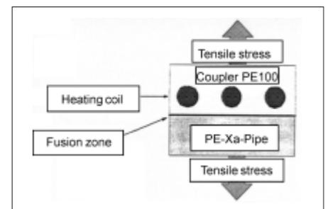
**Fig. 4:** Test sample from the electrofusion zone: tensile test of fusion zone between pipe and coupler
