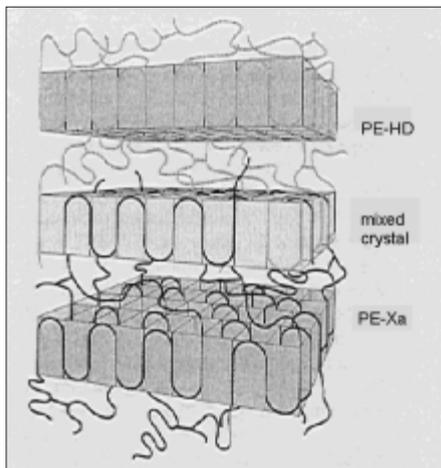
**Fig. 2:** Mixed crystal layer in the fusion zone between HD-PE and PE-Xa [11]
