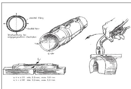
**Fig. 7:** Manual Folding/Bending Test
