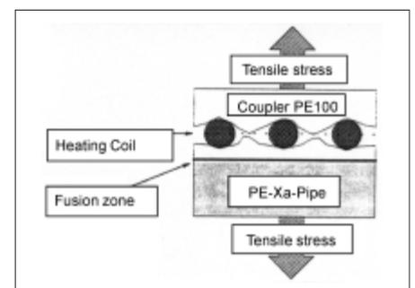
**Fig. 5:** Typical rapture in the coil plane – not in the fusion plane.
