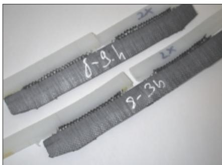
**Fig. 8:** Manuell Folding/Bending test of PE100 Fitting/ PE-Xa-Pipe: Result: Ductile break, high separating forces
