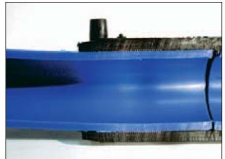
**Illustration 4:** Detail connection zone: bending stresses due to coiled pipes are compensated by the supporting zone
