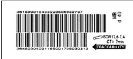
**Illustration 9:** Barcode for fusion parameters and traceability data
